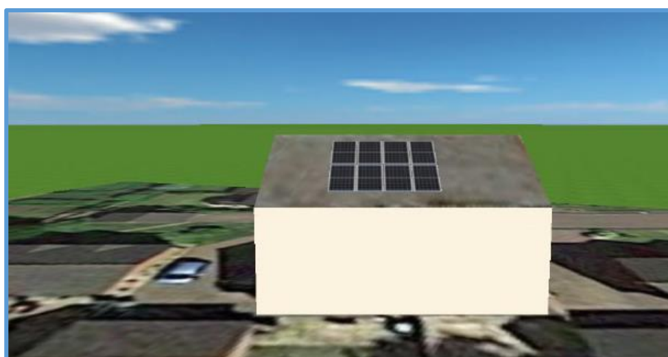
Figure 4.5 – An example domestic rooftop solar PV array of 3kW
